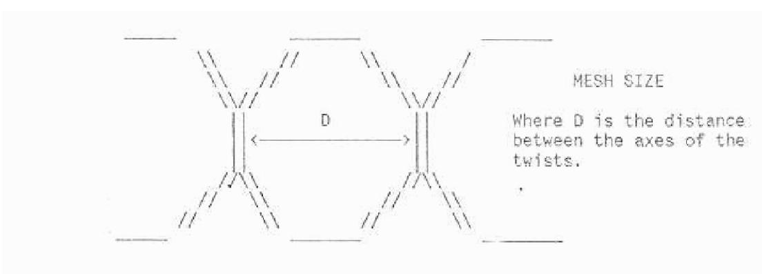
Gabions shall be of the types and sizes shown on the Drawings. The cages shall be constructed from mild steel wire complying with BS 1052, "Specification for mild steel wire for general engineering purposes", galvanised in accordance with BS 443, "Specification for testing zinc coatings on steel wire and for quality requirements". Wire used for the formation of the mesh panel will have a diameter of (2.7 - 3.0 mm). The Properties of Wire for Gabion shall be follows:
